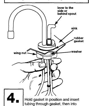
mounting hole. From under sink/cabinet, slide washer then wing nut with flat side facing up over tubing. Check that lever is positioned to the side or behind spout and that spout is positioned to empty into sink. Tighten
